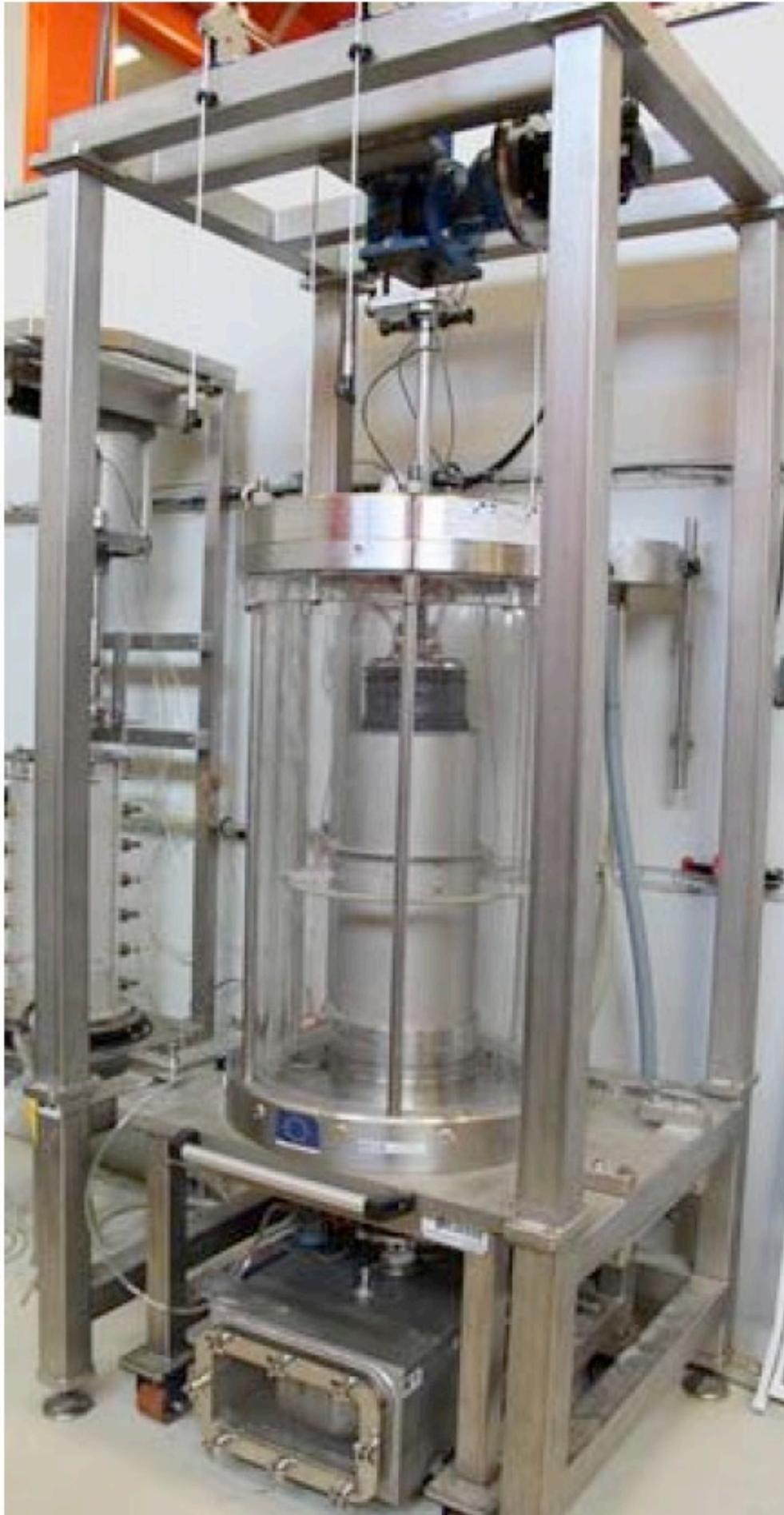
*Figure A.2 – General view of the large triaxial erodimeter*
