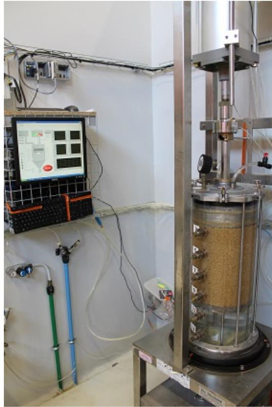
Figure III.2 – Real view of oedo-permeameter
