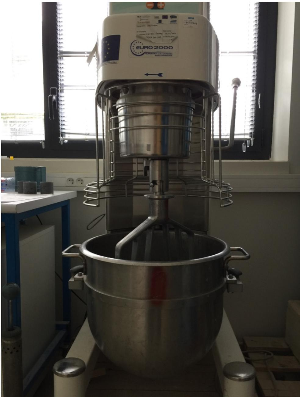
*Figure IV.5 – The electric mixer for production of specimens*
