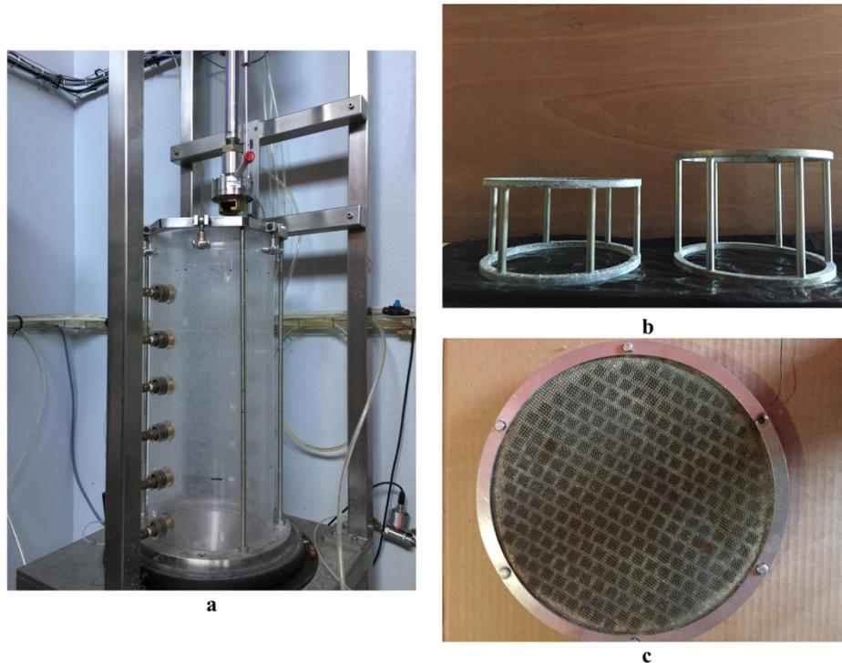
**Figure III.4** – Erosion cell: (a) rigid cylindrical cell; (b) specimen supports; (c) wire mesh and grid
